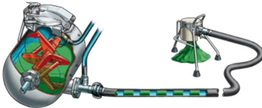
Pneumatic Conveying System
